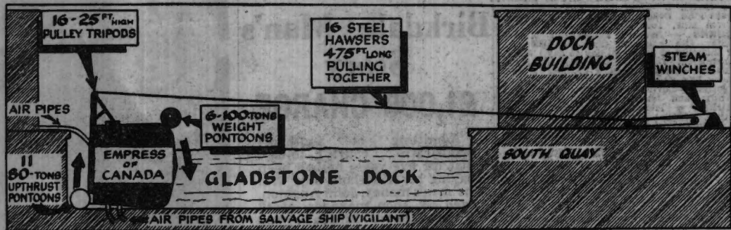
Diagram shows how pontoons, air pipes, and steam winches will be used in to-morrow's salvage operation of the Empress of Canada. (See story on Page Five).
